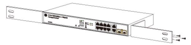
**Step 3:** Secure the brackets tightly, but do not over tighten screws.
